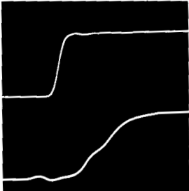
HP 8161A input pulse (upper) and ECL memory output pulse (lower).
